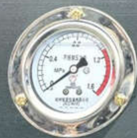
Pump out pressure gauge
